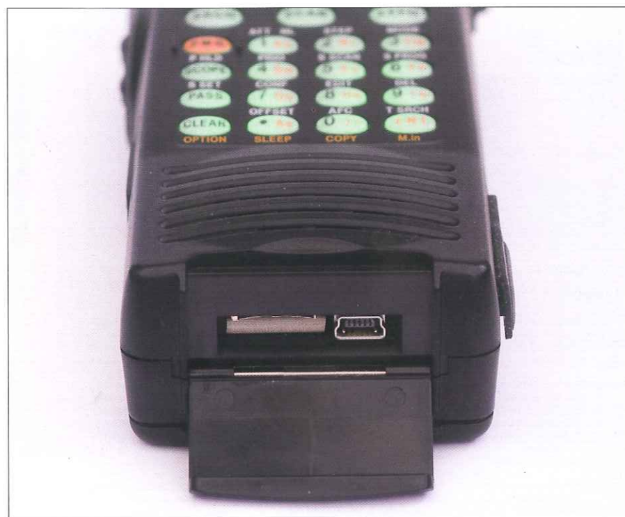
Fig. 4: The micro SD and mini USB sockets are underneath a flap on the bottom panel.
