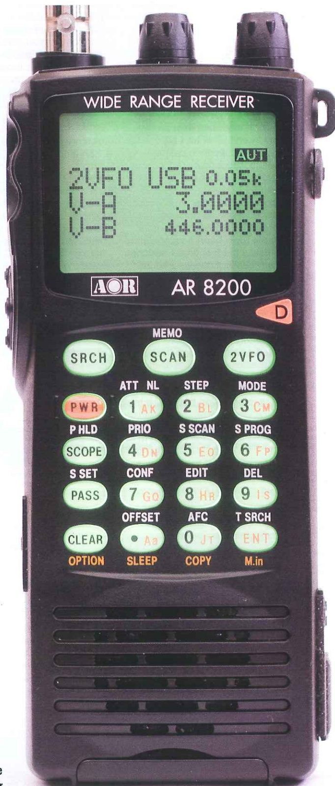
The AOR AR8200D handheld wide range receiver.
