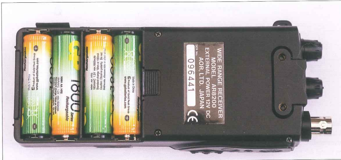
Rear view of the AR8200D with the battery compartment cover removed.
